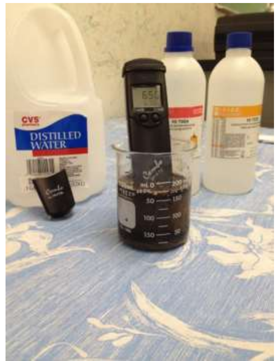
Checking the EC of the water coming out of the hose after the proportioner is a simple way to determine if you are mixing fertilizer correctly and that your proportioner is functioning as it should. Check the fertilizer bag or container for a table of EC readings for target ppm of N at various proportioner settings. The meter in the photo on the right can be used to monitor pH and EC of water and media. Photos: T. Rusinek
