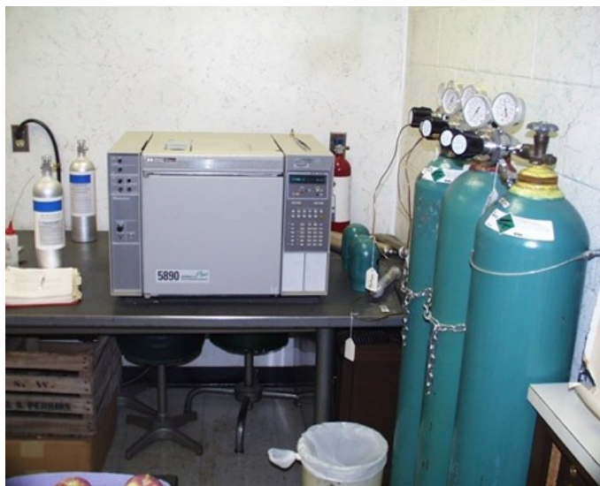
Gas chromatograph at the Hudson Valley Lab, used to measure Internal Ethylene Concentration (IEC).
