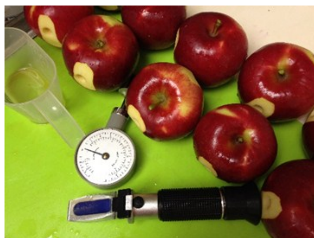
Maturity testing of NY-2 apples. Penetrometer (bottom) measures firmness and refractometer (top) measures sugar concentration. Photo by Amy Ivy.
