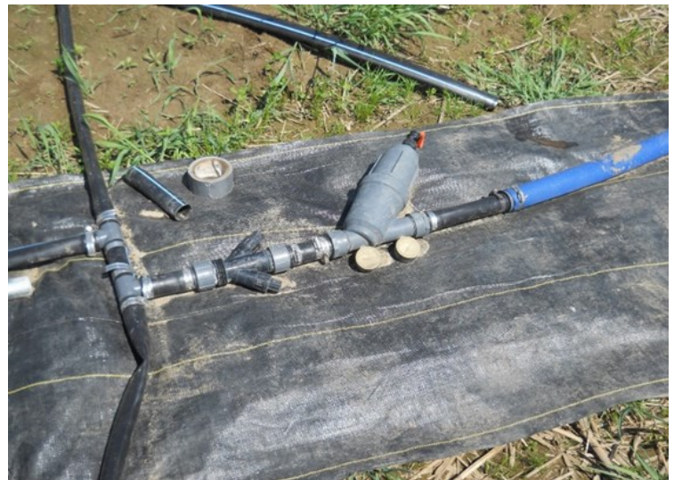
Photo D: Ground cloth under a drip irrigation set-up in the field keeps weeds at bay and the filters, connectors and pressure regulators are easy to reach. Photo ADI
