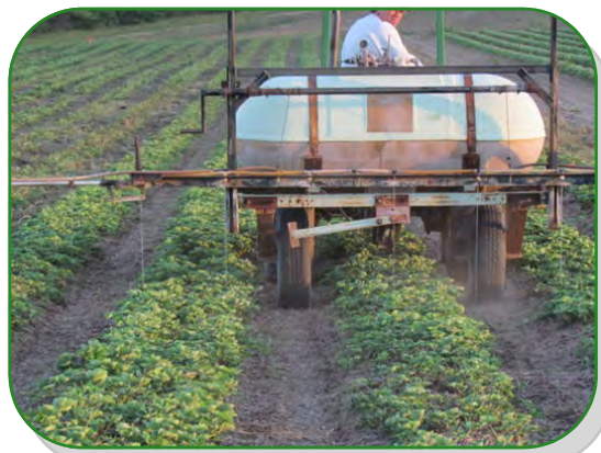
Entomopathogenic nematodes being applied with a normal boom sprayer to a field with Black Vine Weevil problems.
