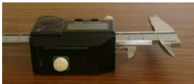
The felt circle (in white) makes the transfer button more tactile Photo by Dan Donahue
