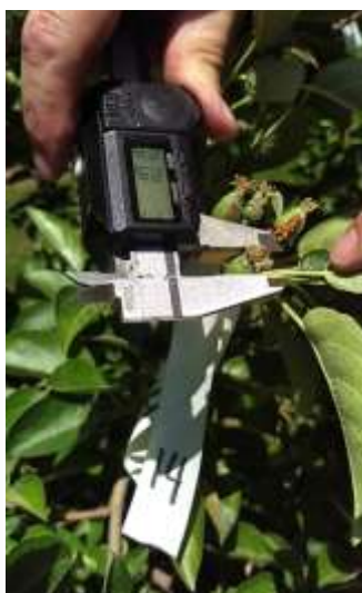
Use of the modified caliper to measure apple fruitlets in a cluster.
