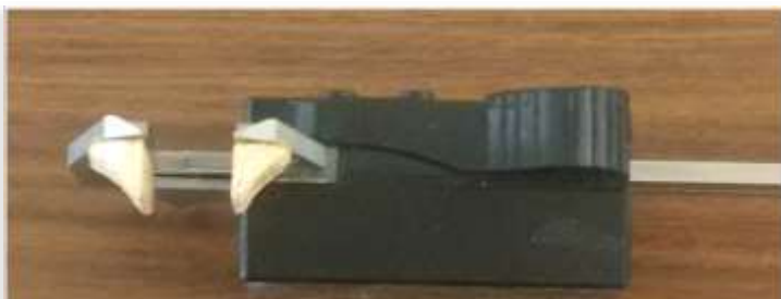
Calipers modified with wooden blocks to increase the available measuring surface. Photo by Dan Donahue
