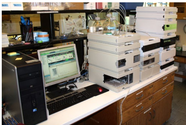
High Pressure Liquid Chromatography (HPLC) unit was used this year to analyze individual acids present in Veraison to Harvest samples.
