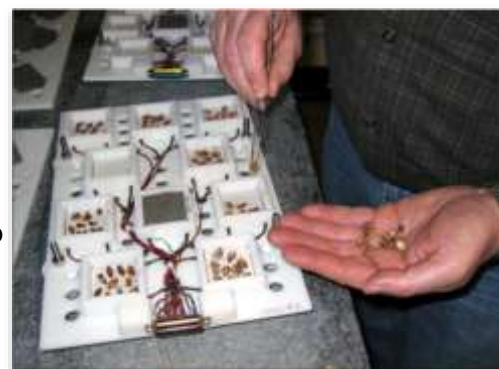
Cut buds are placed on thermocouples in a controlled-temperature freezer to determine lethal temperatures. As buds freeze they release heat, which is detected by the thermocouples.
