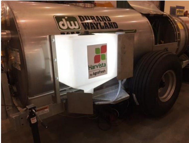
A sprayer with an AgroFresh Harvista nurse tank installed. Photo: Keith Culver, AgroFresh
