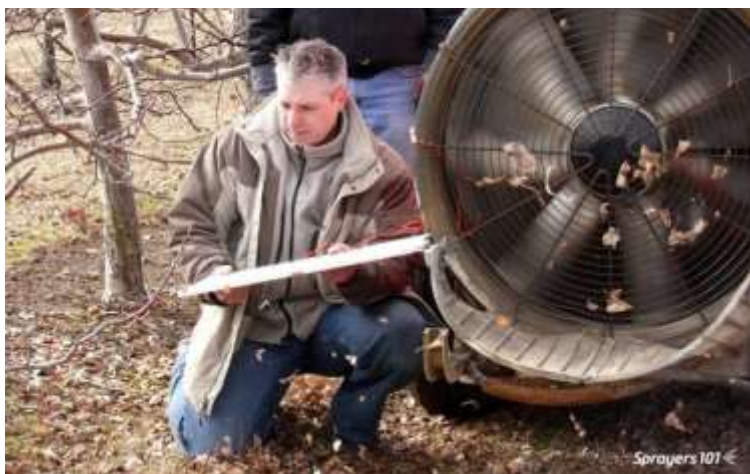
Using a piece of scrap wood with a ribbon on the end to demonstrate how deflectors would channel air on an Economist
