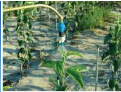
TeeJet ConeJet Nozzle, pressure regulator, swivel head applying 4ML of PGR solution to apple growing tip.
