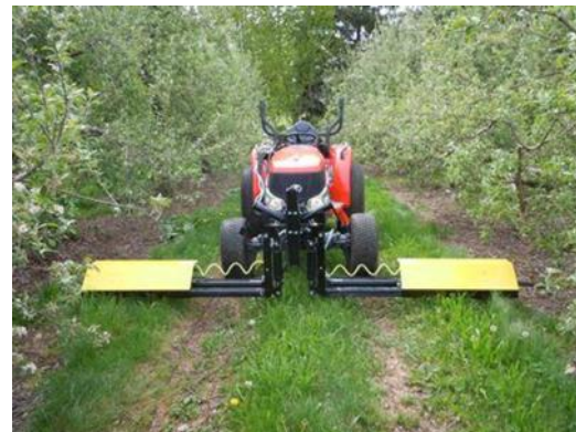
A shielded boom sprayer can minimize herbicide drift to the trees. Photo: Phil Brown Welding.com.
