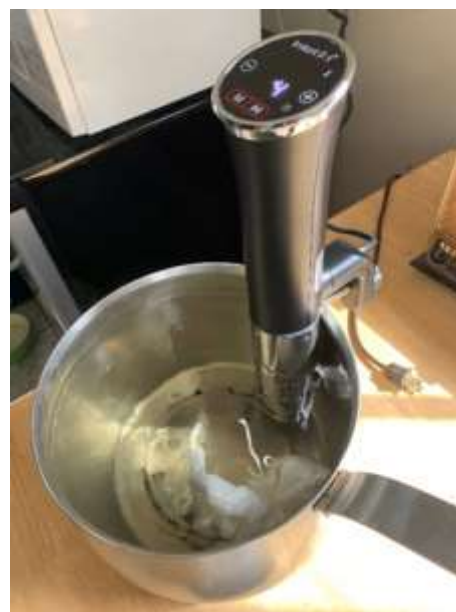
Fig. 1. Sous vide machine heating water for spinach seeds enclosed in a cheesecloth bag.
