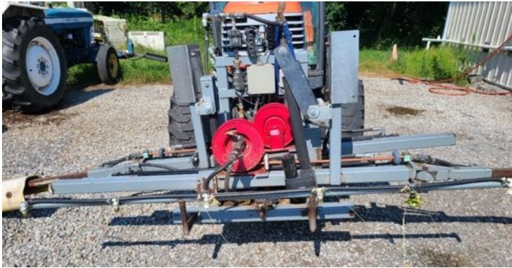
Figure 2. David's sprayer setup. An additional boom is attached to the front of his tractor so he can spray the entire row from tree to tree.
