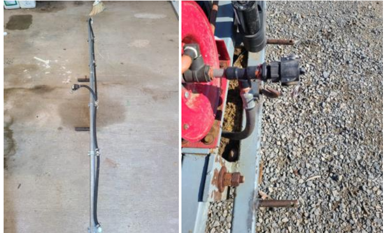
Figure 3 (left). A close-up of the extra boom. Figure 4 (right). The base of the sprayer includes two pins and one quick coupler to attach the front boom to spray the entire orchard floor.
