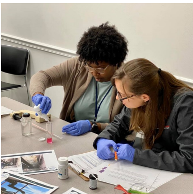
Elisabeth (right) observes post-harvest water chlorine testing using a titration method. Photo courtesy of the Produce Safety Alliance.
