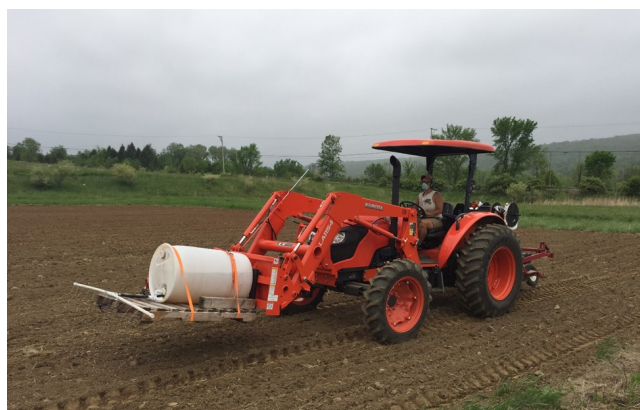
EPN application at Rock Steady Farm in Dutchess County. The gravity fed boom applicator was designed and built by ENYCHP specialists as an alternative EPN application method for farms that do not have spray equipment to cover larger areas.
