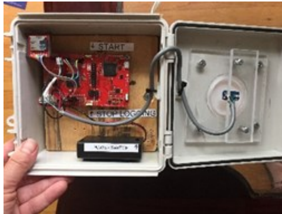
A side-mounted unit containing several light fixtures is passed over a cucumber crop to deliver a disease killing dose of UV-C light. Logger boxes are placed in the crop to measure dosage of each UV-C treatment.
