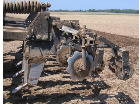
Reduced tiller components (left to right): ripper, fluted coulters and basket. Photo: C. MacNeil, CVP
