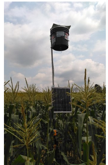
University of Rhode Island Laser Scarecrow design with added solar panel deployed in a field of sweet corn in Rensselaer County.
