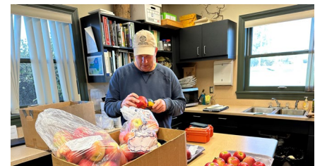
Craig uses a DA meter to measure chlorophyll loss in the fruit peel of an apple. This is a harvest maturity indicator.
