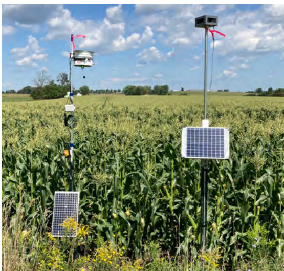
Fields protected with a laser scarecrow (left) plus a Bird Gard® Super Pro distress call system (right) averaged less crop damage than use of either technology alone.
