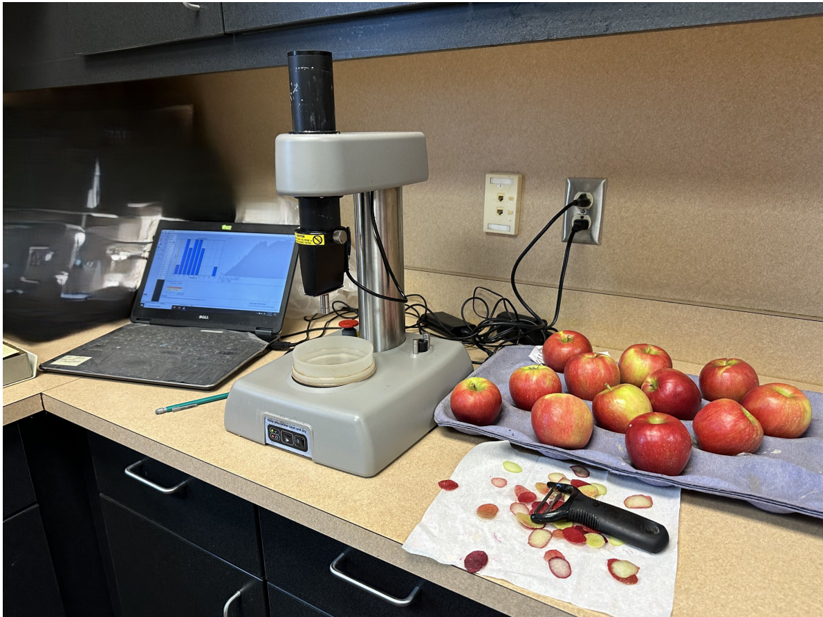
'Fuji' apples awaiting firmness testing with an FTA penetrometer, which measures fruit pressures in lbs./in 2 at the maturity testing lab at Orleans County Cornell Cooperative Extension.
