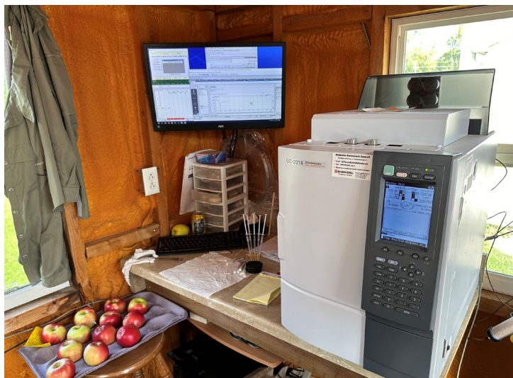
The gas chromatograph at K.M. Davies in Williamson, NY is used to test internal ethylene concentration (IEC) for CCE-LOF’s harvest maturity program. IEC is a maturity indicator for most apple varieties.
