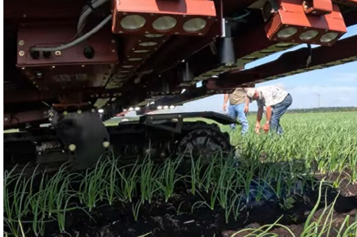
Max Torrey, Big O Farms, Elba and his Carbon Robotics laser weeder (left). It is equipped with 30 x 150 W diode lasers, 42 cameras and 9 LED light panels (right). It is trained using artificial intelligence machine-learning to distinguish between weeds and onions with great precision. Photos by Dylan Sorbello.
