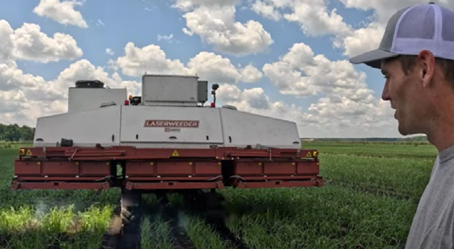
Max Torrey, Big O Farms, Elba and his Carbon Robotics laser weeder (left). It is equipped with 30 x 150 W diode lasers, 42 cameras and 9 LED light panels (right). It is trained using artificial intelligence machine-learning to distinguish between weeds and onions with great precision. Photos by Dylan Sorbello.
