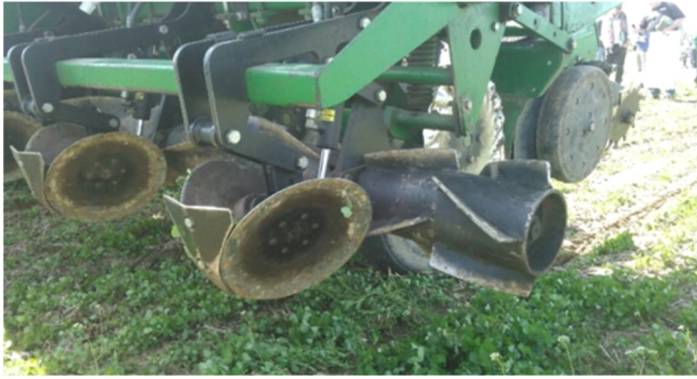
Photo: This is a new “roller crimper” that can be added to any planter to plant into “green cover crops” or any other kind of crop residue. The disks in the front peel away the cover crop or residue and the crimper “crimps” the cover crop to stop it from growing any more.
