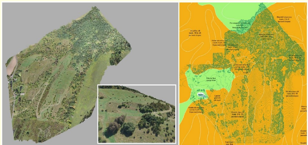
3D interactive model of potential new farm site (left), virtual inspection of a smaller area of the model (inset), and high resolution digital elevation map overlaying the twelve different soil types on the site.
