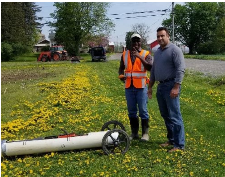
Dr. Oware, University at Buffalo, and Dr. Ali Nafchi, CCE, preparing an electromagnetic induction instrument to gather soil information in a vegetable field which will be used to generate a digital soil map to create management zones in that field.
