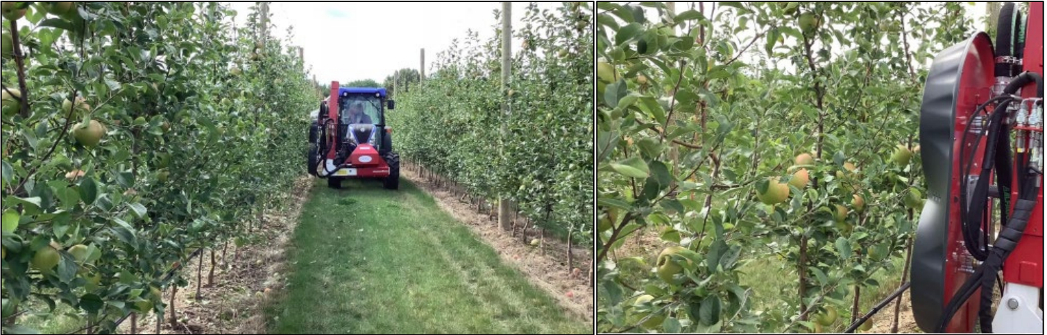
Pneumatic leaf removal machine in action in a young Honeycrisp tree.
