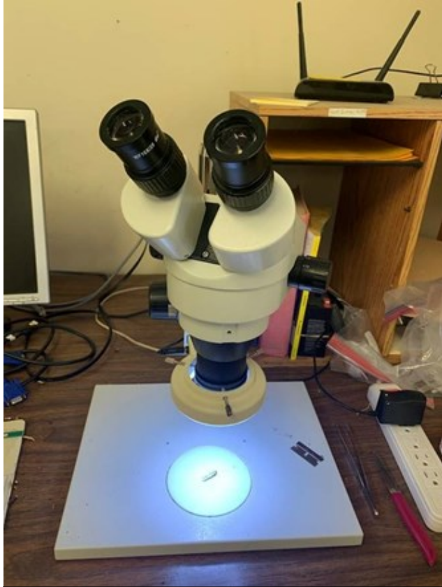
Figure 2. My scope setup. A dissecting scope like this can be purchased online for about $100.
