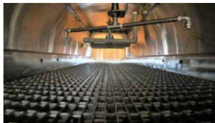
An inside look at the spinning bar and stainless steel conveyor. Photo: A. Chamberlin, UVM
