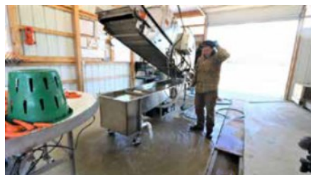
Hinged and lifted via pneumatic cylinders to make cleaning access easy! Photo: A. Chamberlin, UVM
