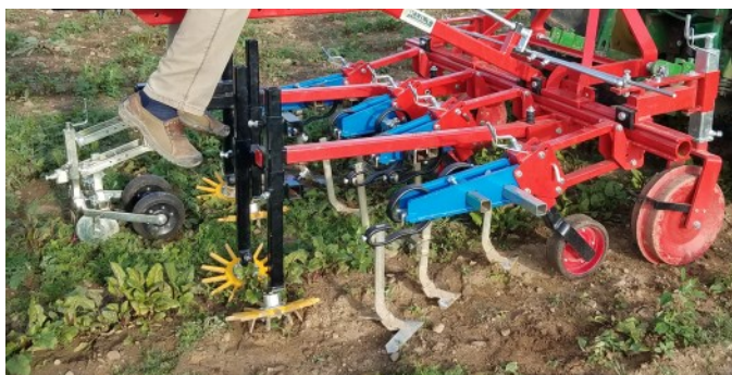
View of between row sweeps with disc on left and fingers on right.
