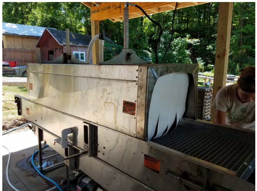
AZS Rinse Conveyor is a stainless-steel produce rinsing machine to aid in the washing of fruits and vegetables. The unit is unique because of the attention paid to the ease of cleaning and sanitizing the equipment after use. Photo by Robert Hadad, CCE Cornell Vegetable Program ●
