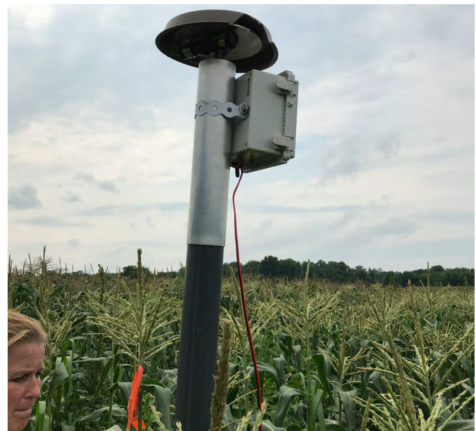
Figure 4. Cornell Cooperative Extension laser scarecrow unit set up in a field. Photo by J. Kikkert, CCE
