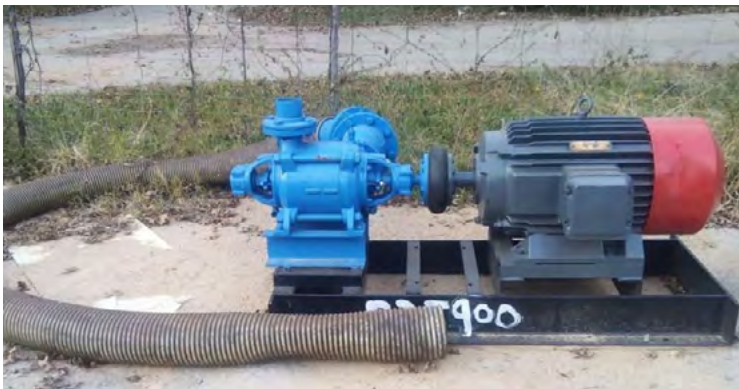
A common type of farm irrigation pump that moves waters into vegetable fields either through overhead sprinklers or larger drip systems. Photo from North Carolina State University Extension.
