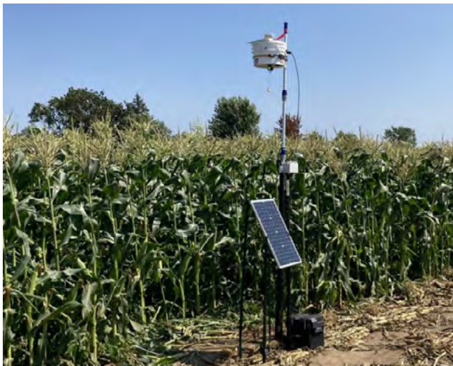
Figure 1. A URI laser scarecrow set up in sweet corn. An optional solar panel keeps the battery charged. Photo: J. Kikkert, CCE Cornell Vegetable Program
