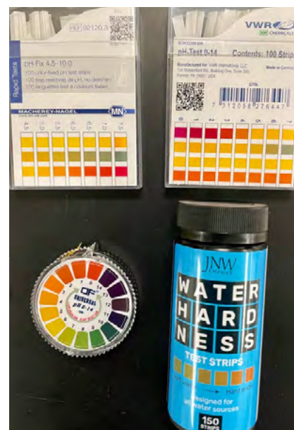
Examples of different pH strips and hardness strips. pH ranges from 0-14 and 4.5-10, hardness range 0-425 ppm. Price is about $10 for 100-150 strips. Photo: Christophe Duplais, Cornell
