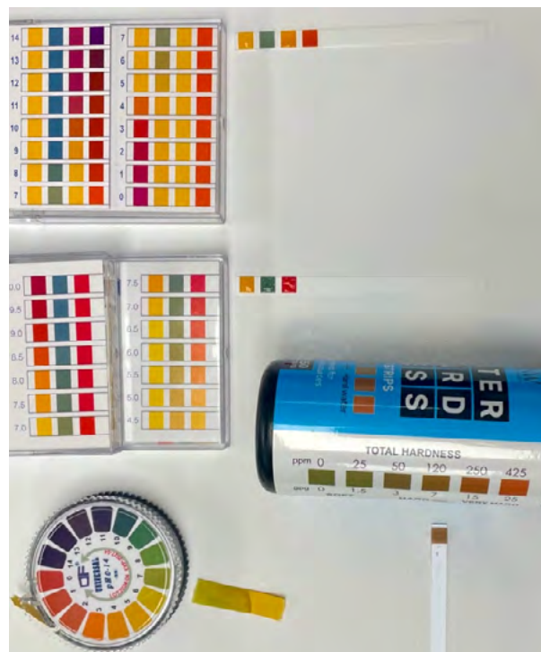
Easy, inexpensive testing of water pH and hardness using strips. Example of readings from sink water at Cornell AgriTech. The pH is between 7 and 7.5 with multicolor strips and between 6 and 7 with paper roll. Multicolored pH strips are more accurate than pH rolls. Water hardness is 7 gpg (120 ppm). Conclusion: This water needs to be treated by buffering and conditioning adjuvants. Photo: Christophe Duplais, Cornell
