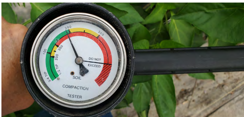
Figure 2. A sample penetrometer reading showing compaction layers in PSI. Photo: J. Reid, Cornell Vegetable Program
