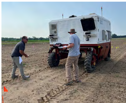
Figure 1. The Carbon Robotics demonstration and research unit in trial at Cornell AgriTech in Geneva. The AI portion of the unit is powered by 12 high-resolution cameras and crop and weed deep learning models. The weeding systems consist of eight 150W CO2 lasers with 3mm accuracy that are ready to fire every 50 milliseconds. Photo: L. Sosnoskie, Cornell
