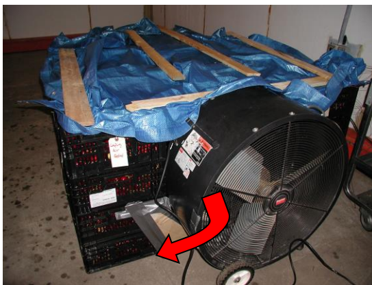
Figure 1. An inexpensive, home -made, forced-air cooling set up
