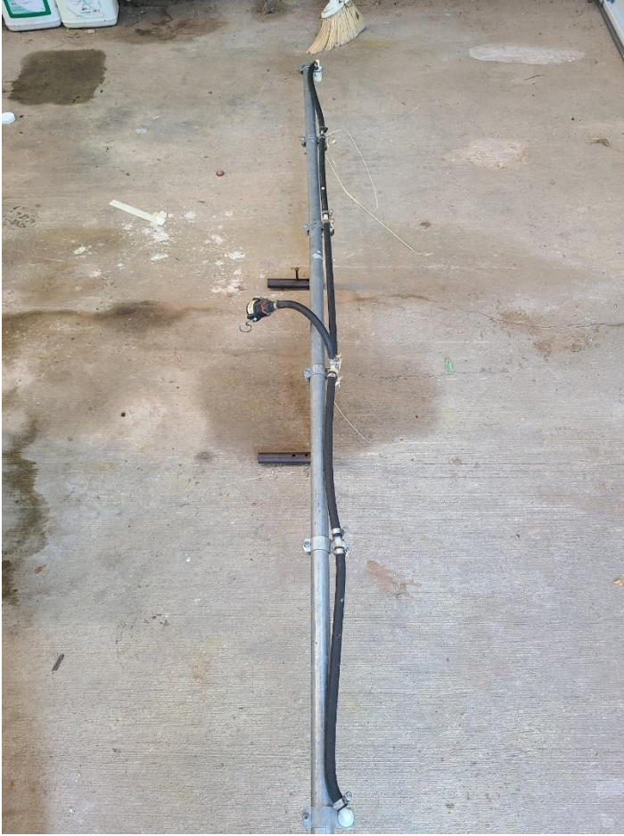
Figure 4. The base of the sprayer includes two pins and one quick coupler to attach the front boom to spray the entire orchard floor.
