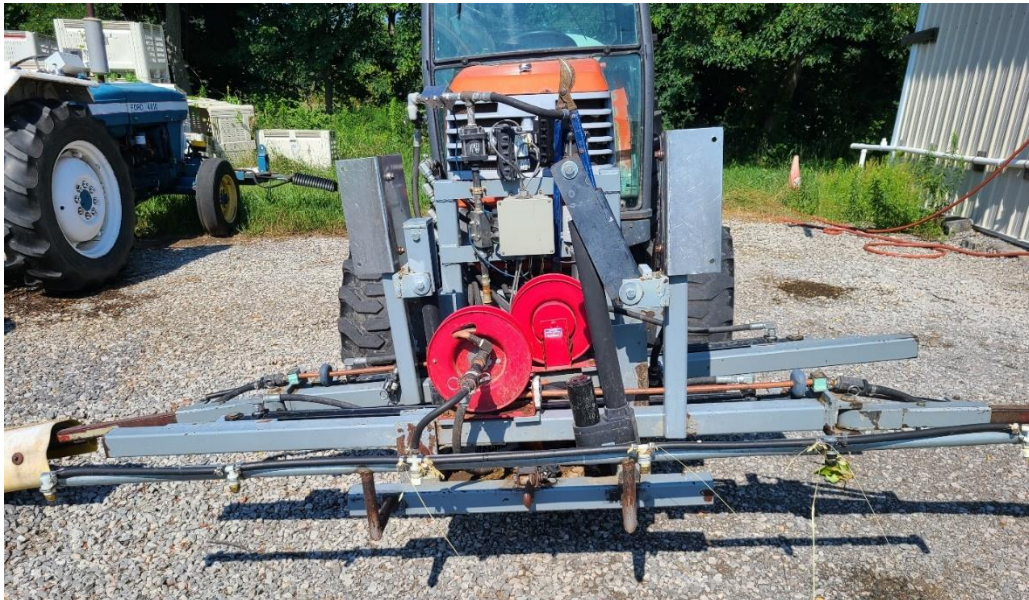
Figure 2. David's sprayer setup. An additional boom is attached to the front of his tractor so he can spray the entire row from tree to tree.
