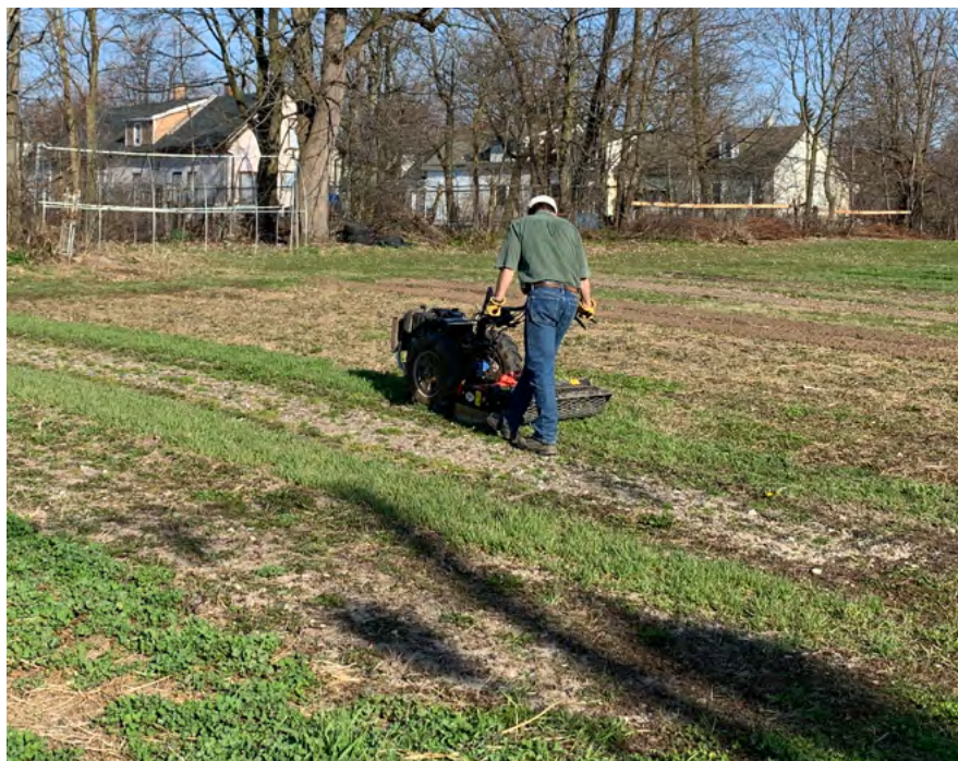
Figure 2. Cover crop incorporation in Spring 2023 using BCS 853 walk behind tractor with a R2 Rinaldi Power Harrow attachment.
