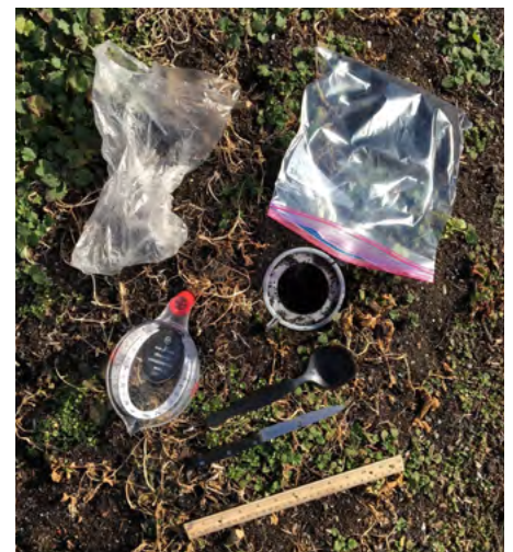
Figure 1. Bulk density samples can be collected without specialized equipment using the “excavation method,” as seen here, or with cylinders designed for this purpose.
