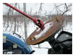
Figure 5. This simple design allowed a worker standing in a platform (not pictured) to drive this tractor and pull a platform for dormant pruning.
