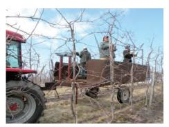
Figure 2. Tractor-pulled orchard platform (designed/built by grower Paul Wafler, Wolcott, NY).
