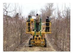
Figure 3. Self-propelled orchard platform (N Blosi from Italy) imported by grower Tom De Marree, Williamson, NY.
