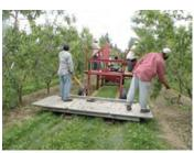
Figure 9. Platform machines can be used for nearly all orchard tasks that ordinarily involve ladders: dormant pruning, trellis building, leader selection, tree training, summer pruning and picking. The use of a platform can facilitate peach harvest (left) and peach hand thinning (right).
