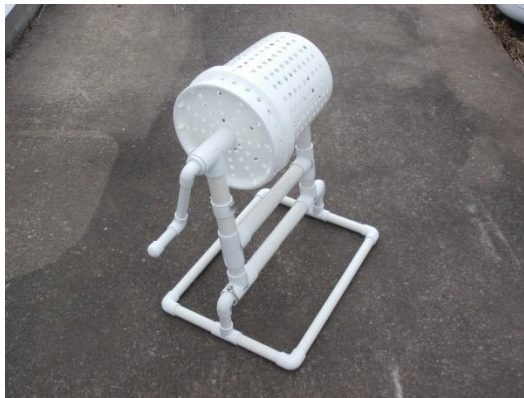
Here is bucket holding arm and bracketing. The bucket mounted onto the brackets and to the stand.
