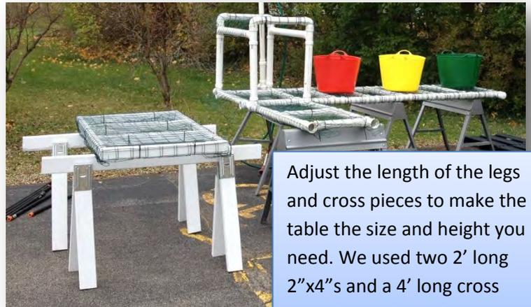
Adjust the length of the legs and cross pieces to make the table the size and height you need. We used two 2' long 2"x4"s and a 4' long cross piece for each sawhorse.
