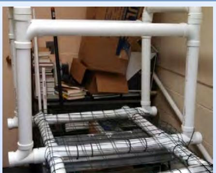
1. Connect T-joints to the 4-way cross connectors using a 2" length of PVC pipe into 4-1" pieces and insert them into the ends of the 4-way cross connectors and the tees as shown in the picture above.
