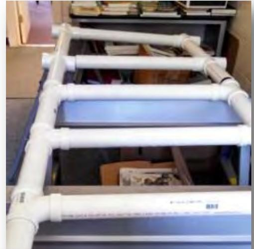
**Tip:** The cross pieces of our frame were slightly wider than the basins. We noticed that the wire fencing sagged when the tubs were filled with water. Doubling of the wire fence top helped reduce sagging of the fence while adding the iron pipes to inside the frame length pieces gave maximum support (but added extra cost).
