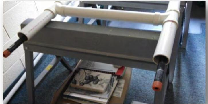
We used coated aluminum sawhorses to support the tabletop. Aluminum won't rust or absorb water making it easy to hose down to clean. Each saw horse is rated to hold over 1000 pounds load. We used three to support the main table, placed so that a cross piece rested on each sawhorse.
