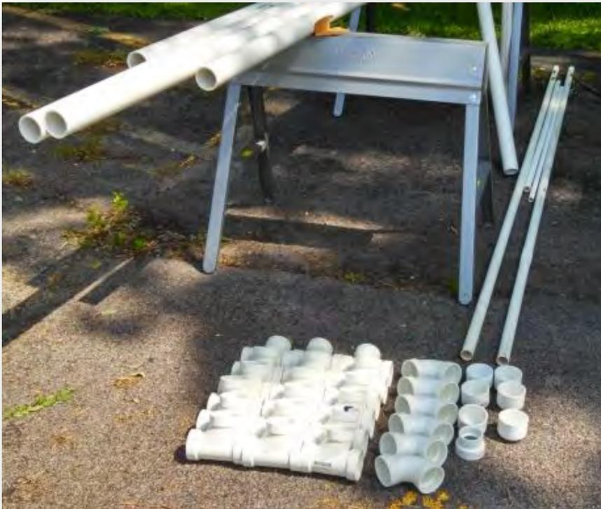
**A simple design:** coated aluminum sawhorses table for the legs, PVC pipes and fittings for the frame and vinyl coated metal fencing for the tabletop.
