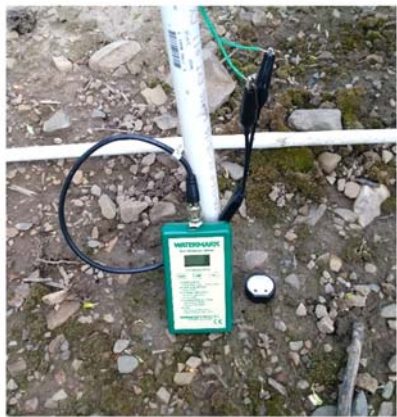
Electronic soil moisture sensor installed in an apple orchard, attached to the electronic sensor reader for measurement.
