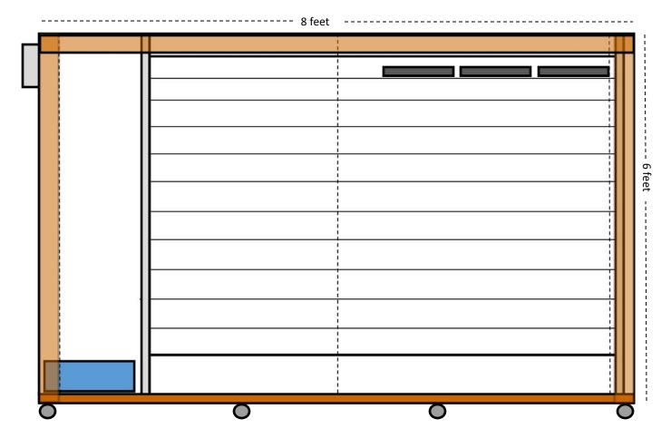
This unit could be easily made to accommodate a variety of spaces, with the box consisting entirely of common lumber. The key technology features of this chamber are the temperature and humidity monitors, which allow the farmer to constantly monitor the chamber despite not living at the farm. Each chamber needs its own monitor, but the cellular relay which conveys information is shared by the two units.
