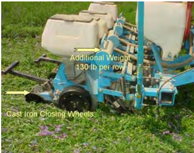
No-till Monosem planter with modifications
