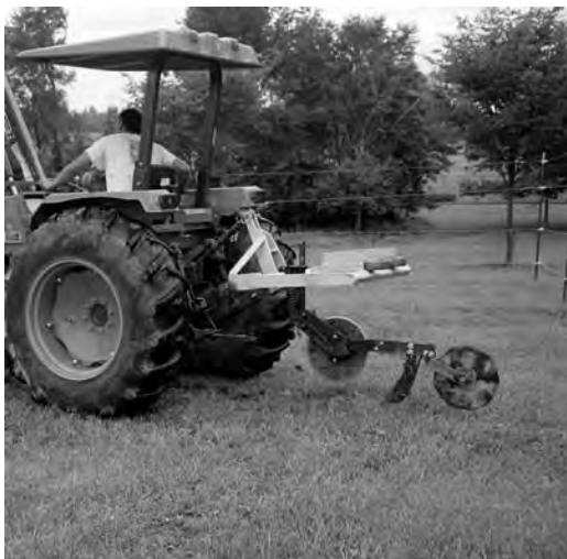
Figure 3. The No-Till Planting Aid (left) prepares a narrow slot in the soil for planting. This snap bean crop (right) was planted in August with a push seeder into furrows prepared with the planting aid. The cover crop residues helped the vegetable by conserving moisture during a hot, dry season.
