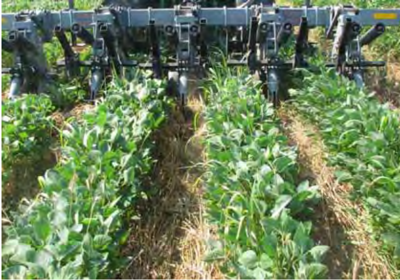
High residue cultivator in no-till soybeans- the rye mat is sliced, but intact
