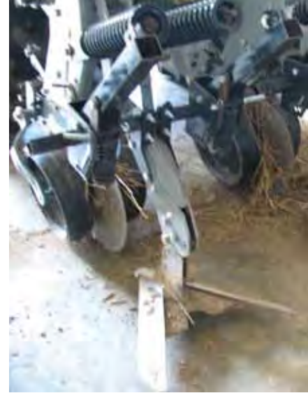
Coulter disc and angled sweep
