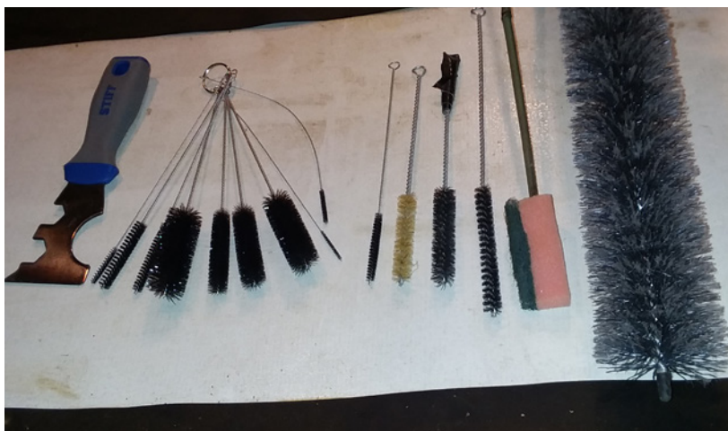
Assortment of tools. From left to right: multi-purpose paint tool, bottle brushes 1/16" – 1", longer handle bottle brushes, scrub sponge on a stick, and dryer vent flex brush. Multi-purpose paint tool is used for getting into tight spaces on the absorber.
