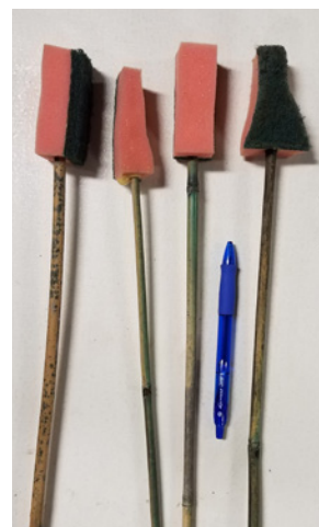
Assortment of custom crafted scrubbers on a stick with various shapes to reach in between rollers, axles, and brushes.
