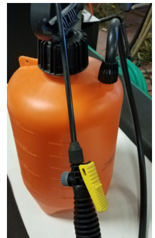
A pump sprayer is ideal for delivering low pressure to specific points that need cleaning. A high pressure washer would splash debris deeper into the equipment, splatter debris onto food contact surfaces all over the facility, and can atomize contaminants that can cross contaminate elsewhere.
