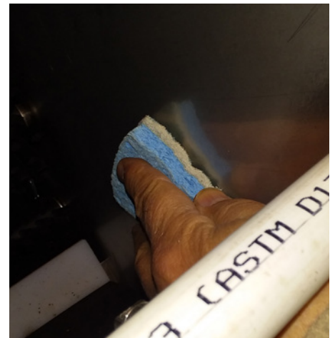
Scrubber sponge should be used for wiping inside and outside walls, wherever reachable.
