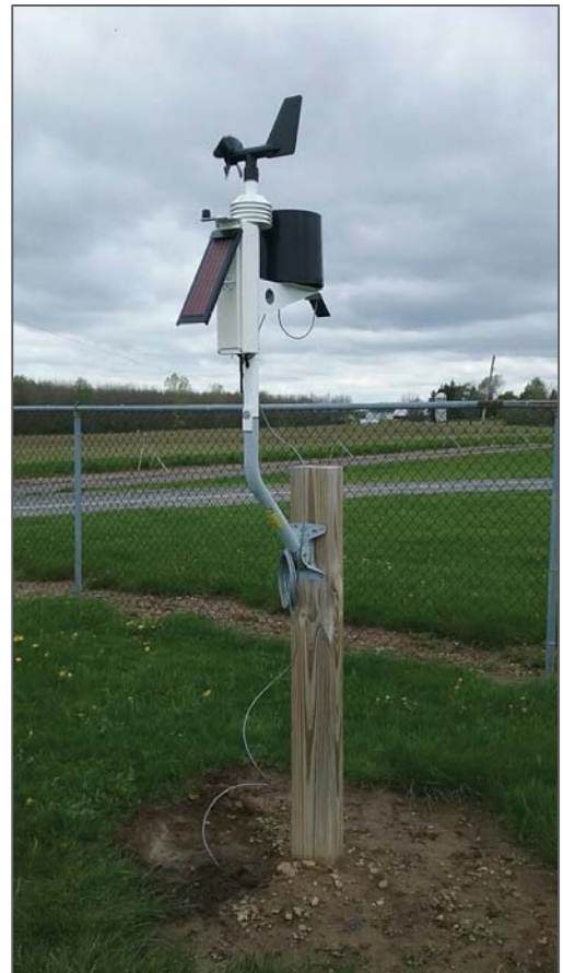
The Rainwise MKIII SP1-LR weather station, located on a Cornell AgriTech @ NYSAES research farm in Geneva, NY. Photo credit: Nicole Mattoon, NYS IPM Program.
