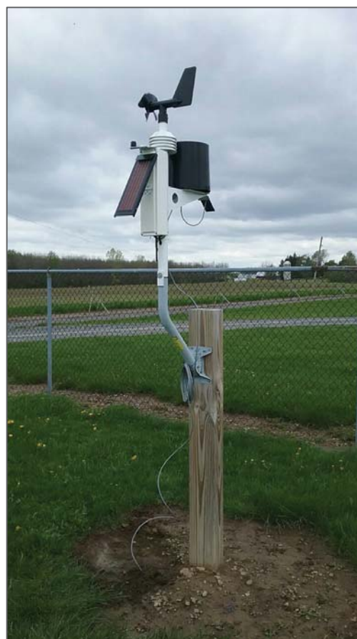
The Rainwise MKIII SP1-LR weather station, located on a Cornell AgriTech @ NYSAES research farm in Geneva, NY. Photo credit: Nicole Mattoon, NYS IPM Program.
