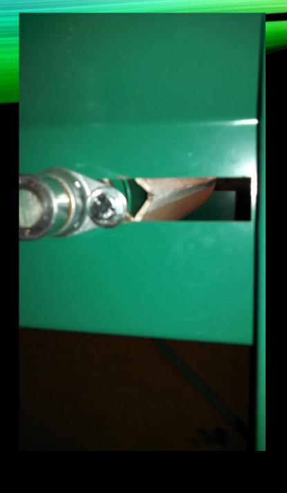
REMOVE CONNECTING ROD FROM SPLICER
