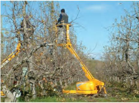
**Figure 1. Single-worker positioning machines (Hydralada from New Zealand) used for dormant pruning of low and medium density orchards.**
