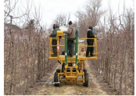
**Figure 3. Self-propelled orchard platform (N Blosi from Italy) imported by grower Tom De Marree, Williamson, NY.**
