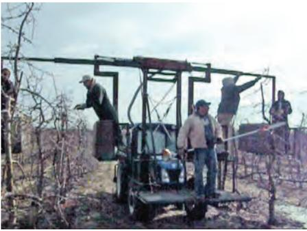
**Figure 4.** Self-propelled two-row orchard platform (designed/built by grower Paul Wafler, Wolcott, NY). A five-man pruning crew is using a self-propelled two-row platform. The worker in the middle makes all big cuts with a pole chainsaw from the moving platform.
