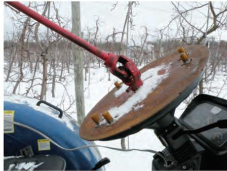
**Figure 5.** This simple design allowed a worker standing in a platform (not pictured) to drive this tractor and pull a platform for dormant pruning.
